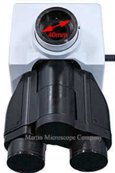
Nikon Eclipse LV100 with 40mm ID Photoport. Requires Nikon MBB63430 to convert to standard 38mm ISO port for use with DxxNLC C-mounts. MDSLR-NK fits this port directly. This is the new Nikon standard port for materials and stereo microscopes.
