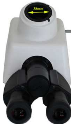
Nikon E200 with non-ISO 38mm port. Requires Nikon MBB73520 Y-T TV Tube for use with DxxNLC C-mounts. MDSLR-NE fits this port directly.
