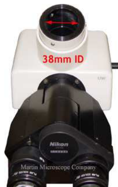
Nikon Labophot-2 ISO 38mm Photoport with "chimney" tube removed. Uses DxxNLC C-mounts. Uses DD20NLT ISO T-mount.
