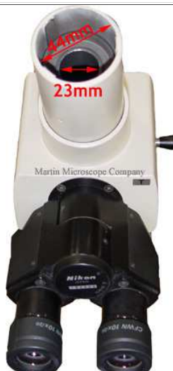
Nikon Optiphot / Labophot "chimney" type phototube with recessed 23mm ID port. MM-SLR, MM99 and MMC00L and variants fit this chimney tube directly; MM3 does not. Uses SCxxNF C-mounts.
