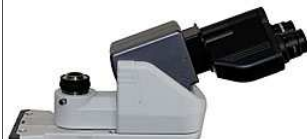
Nikon Eclipse 55i with Ergo Head and built-in 0.7x C-mount Phototube.
