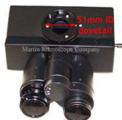
Olympus BX with 51mm ID dovetail Photoport. Uses DxxBXC C-mounts. MDSLR-BX fits this port directly. Also for Olympus SZX.
