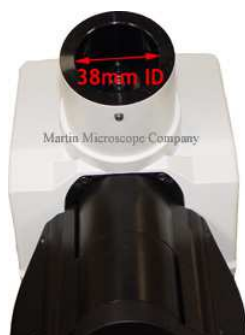
Nikon Eclipse with ISO 38mm ID Photoport - Nikon "chimney" tube has been removed. Uses DxxNLC C-mounts. Uses DD20NLT ISO T-mount.
