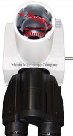
Nikon Eclipse with "Chimney" phototube with recessed 30mm ID port. MM-SLR, MM99 and MMC00L and variants fit this chimney tube directly; MM3 does not. Uses SCxxNF C-mounts.
